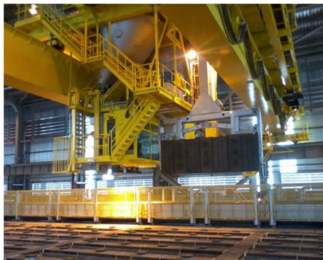
Figure 4. View of an FTA crane handling a batch of anodes.
