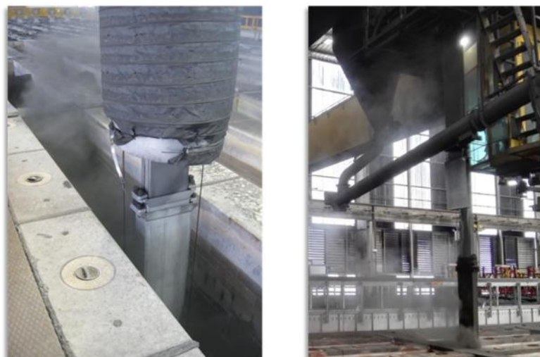
Figure 7. Present dust suction system. Left: local suction device, Right: Dust emissions as observed.
